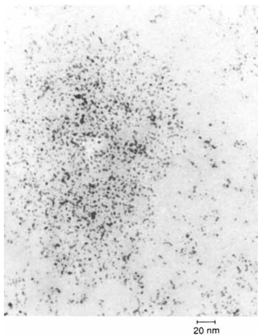
Fig. 1 Typical electron micrograph of palladium nanoparticles [ex-Pd-MeC(O)Et-KD1] dispersed on lacey carbon film, magnification 200 K
